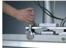
The blade is easily changed within 2 minutes
